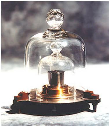
K48 [here to the left] came from the second batch of kilogram replicas to be produced. It was delivered to Denmark in 1949 with an official mass of 1 kg+81 µg. Like all other replicas, it is stored under two nested bell jars virtually all the time. Still, its mass and that of the IPK diverged markedly in only 40 years; the mass of K48 was certified as 1 kg+112 µg during the 1988–1992 periodic verification.
